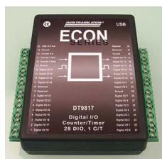
2.0 bus. The DT9817-H furnishes 28 programmable digital I/O lines and can sink 64 mA or source 15 mA at standard logic levels. Simply install the supplied GO! software, connect your signals to the screw terminals of the module, and plug the module into the USB port of your computer. For more advanced applications, the module also ships with extensive software tools, including DTx-EZ for Visual Basic or Visual C++, DT-LV
