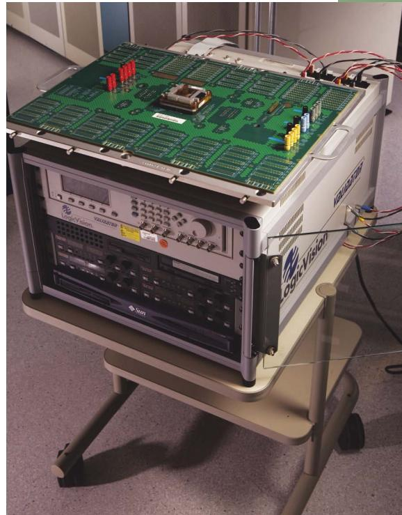
A modified board employs banana jacks and other connectors to provide a Validator benchtop system with access to power and ground planes, high-speed clocks, and the test access port.
