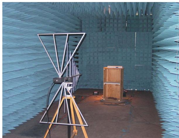
An EMI chamber lets DPS engineers perform precompliance tests in house. Courtesy of DPS Telecom.
