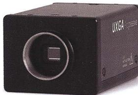
The top-of-the-line model, the XCL-U1000 black-and-white camera, measures only  $1\frac{3}{16}$  in. by  $2\frac{1}{16}$  in. by  $3\frac{3}{16}$  in. and incorporates a  $1/1.8$ -type progressive-scan CCD that produces detailed, ultra extended graphics array (UXGA) resolution images (1,600 by 1,200 pixels) at 15 frames/s.
